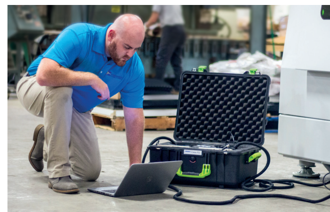
Vibration measurement on site
