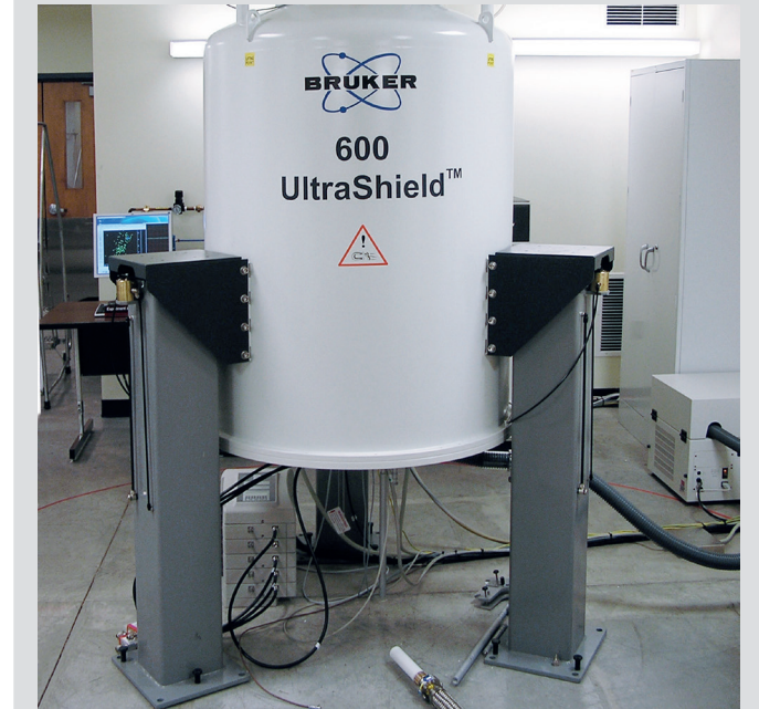
600 MHz NMR on PAL18 gimbal air springs
