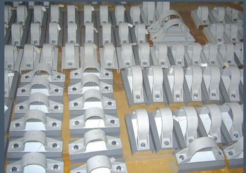
Fabricated pipe clamps for petrochemical pipe application.
