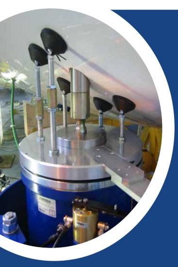
Professionals can save time and money during GVT by using a Fabreeka custom SSS. Traditional methods — such as testing with bungee cords — are very time-consuming. Bungee methods require adjustments and reconfigurations for every load condition, which adds both time and cost to testing. Also, older systems may require dangerous critical lifts where cranes must lift the plane for the isolators to be installed under the aircraft.
