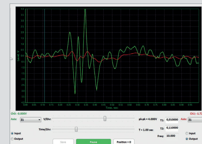
Real-time vibration measurement by oscilloscope
