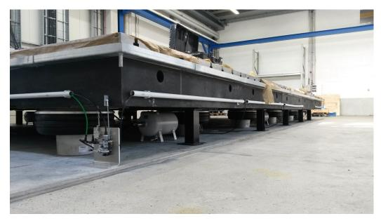
Pneumatic isolators provided by Fabreeka also support applications with large dynamic displacements and where lift height is required as in this hydropuls test rig for trucks.
