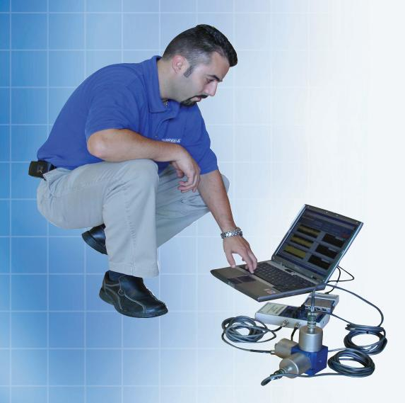
Low frequency vibrations can adversely affect the accuracy, repeatability and throughput quality of your machine tool. A vibration site survey/analysis will determine the levels of vibration existing at your site which is required for proper vibration control recommendations to be made.
