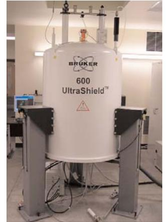
Above right, isolators for NMR magnets can be 42" to 72" in height and have vertical and horizontal natural frequencies as low as 0.8 Hz.
