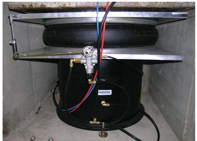
Single convolution air bag isolator with damping chamber and leveling valve supporting a reaction mass for electrodynamic shaker.
