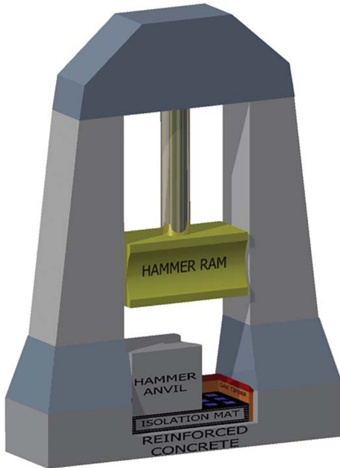
Forging hammer installed on concrete reaction mass supported by Fabreeka isolation mat.
