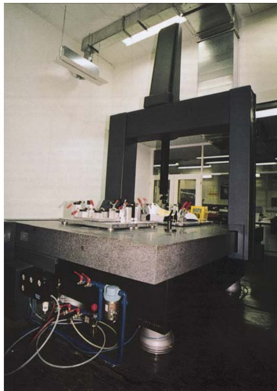
Vibration isolators stabilize floor vibrations for coordinate measuring machines, increasing CMM accuracy and repeatability.
