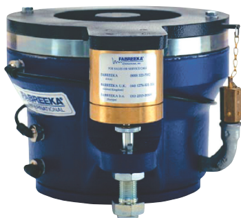
A standard pneumatic isolator has a natural frequency of approximately 2.5 Hz. These isolators require a source of clean, dry gas with pressures from 60 to 120 psi.
