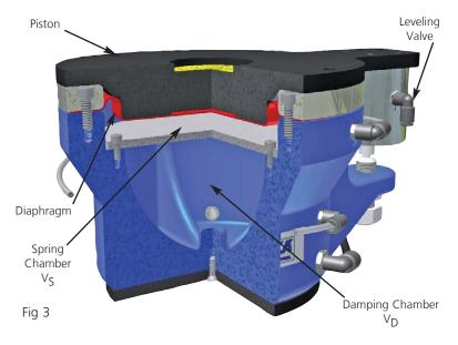
The effective area of the diaphragm and the pressure on the diaphragm define the load capacity of the isolator. The pressure in the isolator is controlled by a leveling valve that controls both the internal pressure and "float" height of the isolator.
