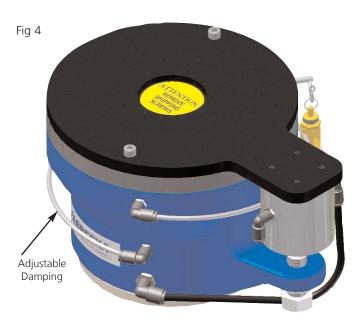
Damping is looked at carefully to give the best effective isolation that can be achieved. For air spring-mass systems, damping is essential to stop transient vibrations following a disturbance such as a stage or bridge moving and to limit the amplitude of forced vibration at the isolator's natural frequency. The length and diameter of the tubing are chosen for a given volume ratio to create laminar flow in the damper. This design concept
