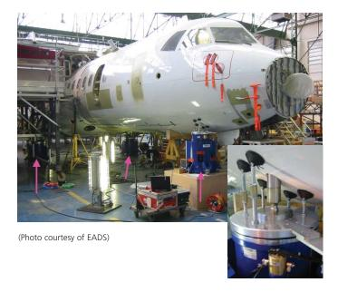
Isolators used for GVT have vertical and horizontal natural frequencies as low as 0.5 Hz.
