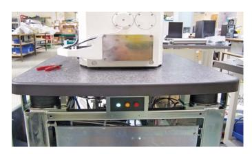
PLM-3 mounts are integrated into the frame of Carl Zeiss EVO series SEM microscopes. The chamber and column are isolated to provide greater than 300,000 times magnification for X-ray geometry and electron imaging.
