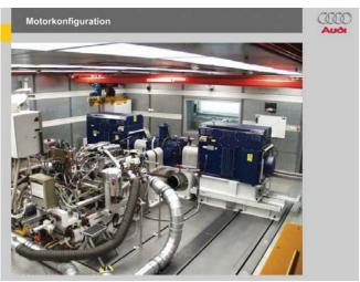
Engine/dynamometer testing on bedplate and support foundation.
