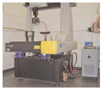
Delta K pneumatic isolation system module allows the Brown & Sharpe Global 7.10.7 CMM to operate at its designed speed and accuracy when supported on pneumatic isolators.
