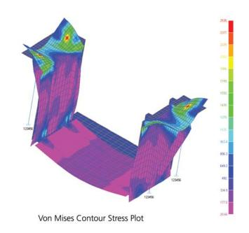
Fig 12 Stress analysis of a steel support frame for an electron microscope. The frame will also be analyzed dynamically for structural modes (resonances).
