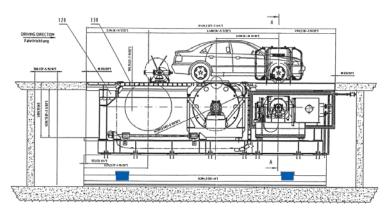
Rolling road test equipment on isolated support foundation
