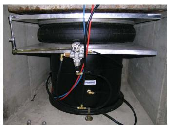
Single convolution air bag isolator with damping chamber and leveling valve supporting a reaction mass for electrodynamic shaker.
