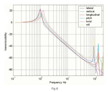
Transmissibility curve showing isolator translational and rotational frequencies, as well as support/machine base structural modes (resonances) above 80 Hz.
