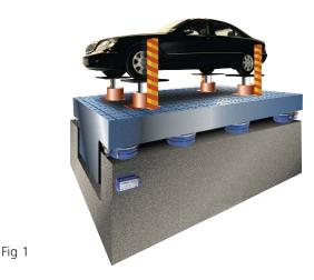
A four-post road simulator test rig creates high amplitude vibration and shock at low frequencies to test vehicles for "squeak, rattle and roll" conditions. Pneumatic isolators reduce the vibration and shock transmitted to the environment.
