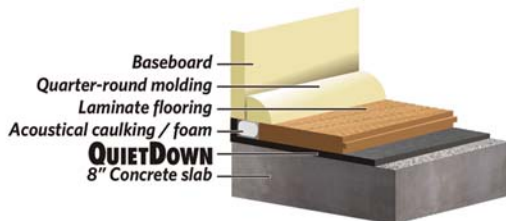
Concrete slab with floating laminate
