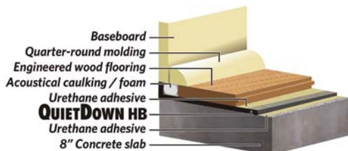
Concrete slab with engineered wood
