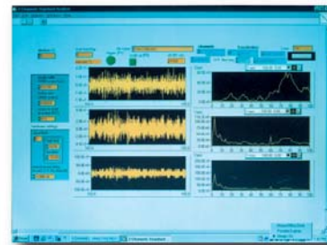
Vibration measurement software records amplitude and frequency data for analysis.
