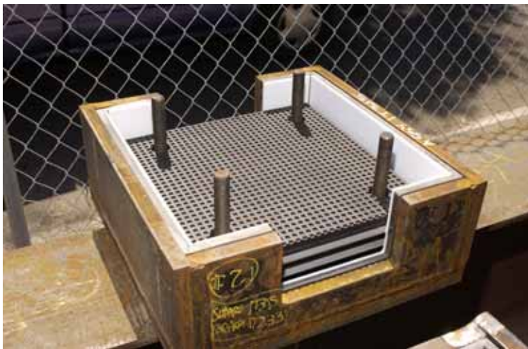
Isolators made of twelve layers of Fabcel pad with three shims are used to control stability and expansion on deflection. PTFE covers the inside of the “box”, to insure no binding when the pad deflects and returns to its original position.
