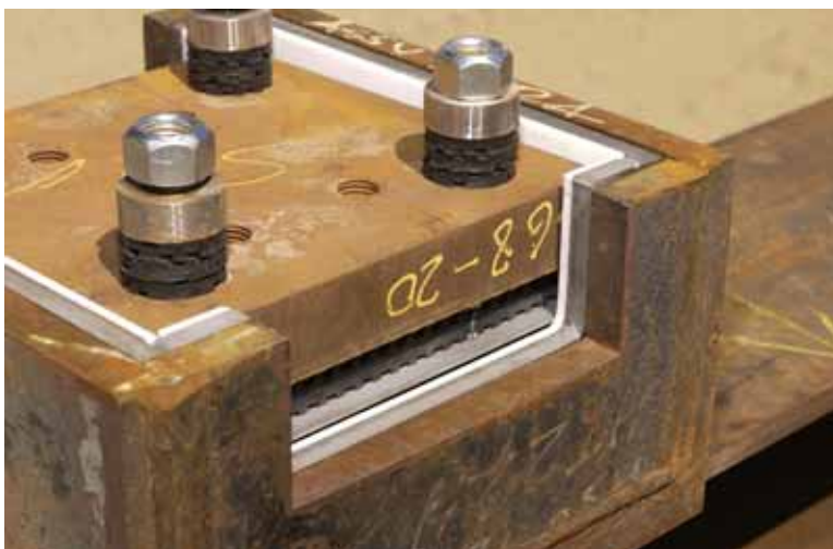
Fabcel washers are used to isolate the fastener so there is no transmission of vibration.
