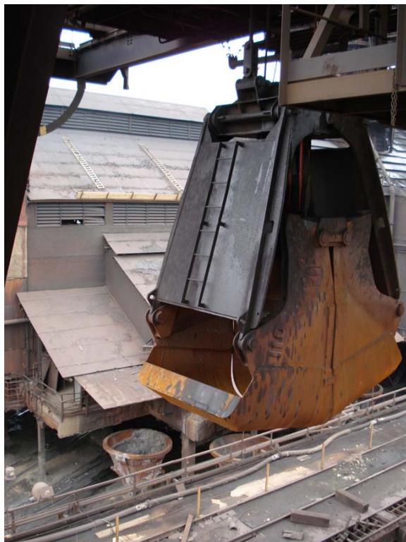
The clam bucket (at left) that scoops the ore pellets weighs approximately 20 tons when full. This is attached to the trolley that moves over the rail (below).
