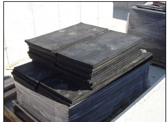
Fabcel mounts prior to installation.
